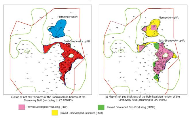
Fig. 6. Comparison of categorization of reserves according to the Russian classification (a) and according to PRMS (b)
