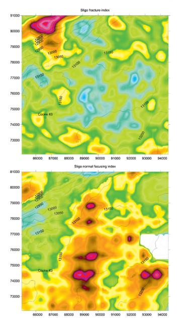
Fig. 11. Open fracture intensity (top) and oil-bearing capacity (bottom) slices along the Sligo structural horizon
