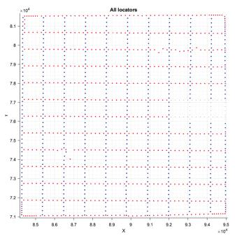
Fig. 10. CDP-3D seismic survey standard acquisition system (receiver points are shown in blue, shotpoints are shown in red)
