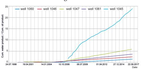
Fig. 1. The graph of the accumulated water-oil factor showing the well with the presence of technogenic filtration channel
