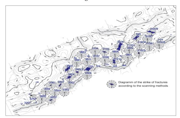
Fig. 9. Evaluation of the dominant direction of the strike of fractures in the studied reservoir along the horizontal
