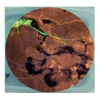
Fig. 2. Caverns along the fractures, (with bitumen)
