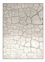
Fig. 1. Formation of a block structure under biaxial tension conditions (Revuzhenko, 2000)
