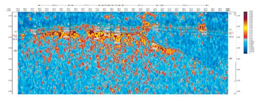
Fig. 7. Time section of scattered waves through wells. Identification of healed faults and faults with open fracturing
