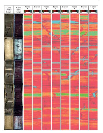
Fig. 6. Photo of core and processing of FMI primary data ("POMOR-GERS") for further analysis with a high evidence base
