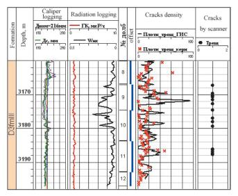
*Fig. 11. Comparison of fracture density, defined according to the sonic log data and on a core column*
