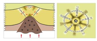
*Fig. 6. Tectonophysical model of fracturing and compaction zones distribution on an anticline structure in vertical section (left) and horizontal section (right)*
