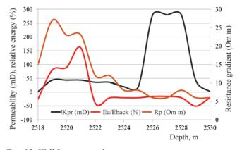
Fig. 13. Well Logging and seismo-acoustic emission energy
