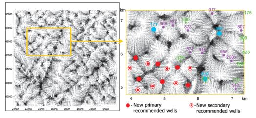
Fig. 5. An example of a reservoir mini-block structure created by diagonal and radial fracturing systems, and its enlarged fragment with recommended well locations (on the right) according to the fracturing field vector-gradient obtained by MSE waves and SLEC technology. Reservoir depth of about 4 km, Rostashinskoye field, Orenburg region
