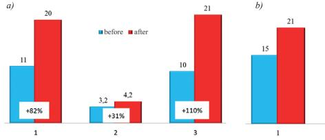
Fig. 5. The change in the permeability of the reservoir during the process of acoustic impact. a) Permeability of the bottomhole zone (mD); b) Permeability of the remote zone (mD). 1 - well No. 174 of the Pikhtovsky field, 2 - well No. 266 of the Olkhovsky field, 3 - well No. 255 of the Unvinsky field
