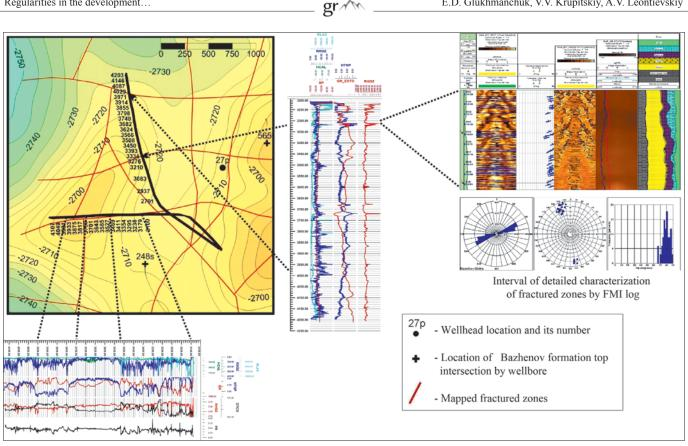
Fig. 5. Fracturing zones in the rocks of the Bazhenov formation according to horizontal well logging data
