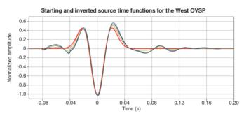
Figure 3. Source time function for the  $4^{th}$  inversion of the West OVSP data. The starting wavelet is denoted by the thick red line while the thin orange, green, blue and black lines denote respectively the inverted wavelet at iteration 5, 20, 50 and 100.
