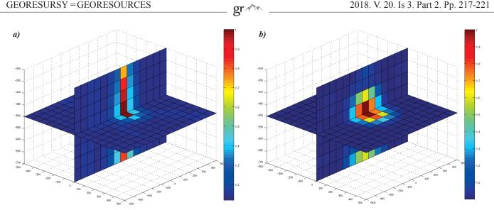
Fig. 2. Accuracy of localization of the model microseism by the methods of Capon (a) and maximum likelihood (b) in space for a low noise level
