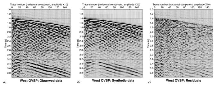
Figure 2. Horizontal component of the West OVSP data. Low-pass filtered observed data (corner frequencies of 20 and 40Hz), synthetic data and residuals are displayed respectively at left, on the middle and at right. The fit between observed and synthetic is fairly good providing low residuals (remaining misfit is 20%). Structured energy in the residuals shows that some reflected and transmitted S-waves are not fully explained.
