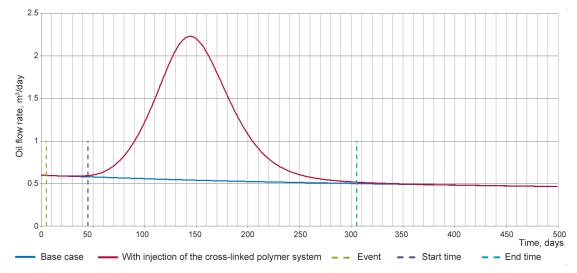
Fig. 5. The prediction of the flow rate of oil obtained from blocking the channel filtration. The blue line in fig. 5 shows the base case. The increase in oil production from injection of the cross-linked polymer system into the injection well is shown by a red line. Dashed lines indicate the time of the event (green), the start time (purple) and the end time (blue) of the resulting effect
