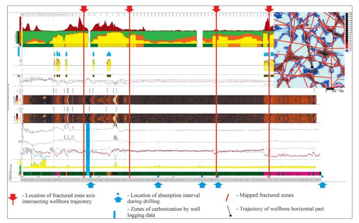
Fig. 7. Fracturing zones in the rocks of the Tyumen formation according to horizontal well logging data
