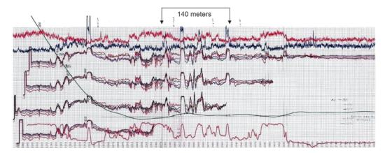
Fig. 4. Fracturing zones in Cretaceous sediments (AS reservoir) according to horizontal well logging data
