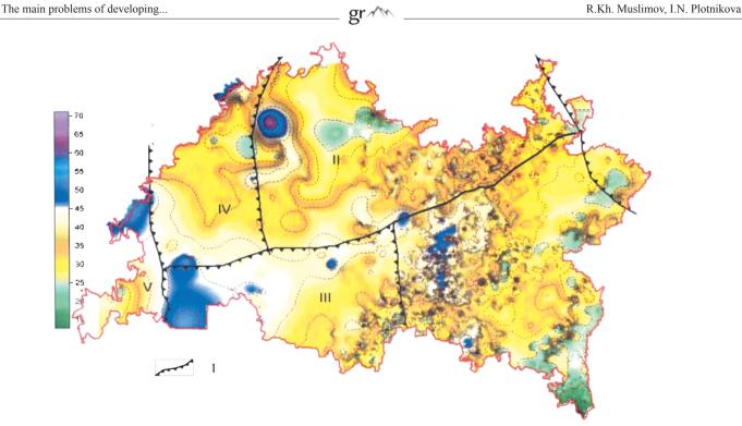
Fig. 2. Capacity map of the Semilukskian horizon of Tatarstan (according to Khisamov et al., 2010). 1 - modern boundaries of the structures of the 1st order; I - South-Tatar arch, II - North-Tatar arch, III - Melekess depression, IV - Kazan-Kazhim aulacogen, V - East slope of the Tokmov arch.
