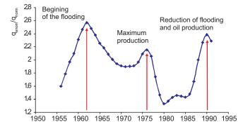
Fig. 1. Dynamics of the ratio of average production rates of anomalous wells to average production rates of normal wells in the Minnibayevsky area over 40 years of their operation (according to Khisamov et al., 2012)
