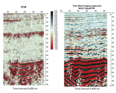
Fig. 15. Example of time sections RTM and MULTI BackRTM
