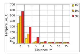
Fig. 2. Estimated levels of temperatures reached in the bottomhole zone at various volumes of BM  $NH_4NO_3/NaNO_3$ , injection
