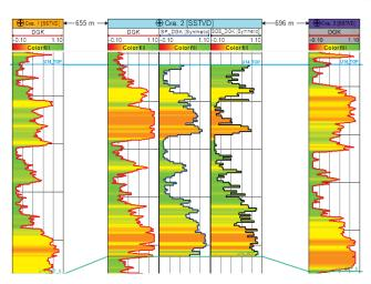
Fig. 2. Comparison of real and synthetic gamma logging curves. DGK, red curve – real logging, SP\_DGK, blue curve – synthetic logging modeled by the spectral method, SGS\_DGK, black curve – synthetic logging modeled by the SGS method.
