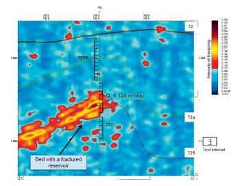
Fig. 5. Time section of scattered waves through well 15
