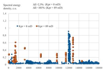
Fig. 4. Discrete range of acoustic emission during fluid filtering (Hz)
