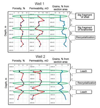
*Fig. 2. Connection of primary sedimentation signs of rocks with their porosity*
