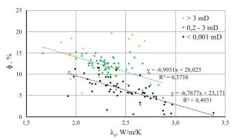
Fig. 6. Collection 2. Connections between porosity and thermal conductivity and linear trends for groups of "poorly permeable", "medium-permeable" and "high-permeable" samples
