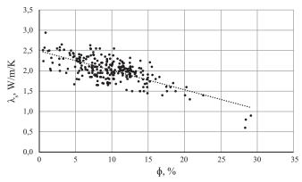
Fig. 5. Linear inverse correlation dependence between the measured values of thermal conductivity ( $\lambda_s$ ) and ( $\phi$ ) of all samples from Collections 1 and 2. Regression equation:  $\lambda_s = 2.49 - 0.05\phi$  ( $R^2 = 0.5$ ; N = 263)
