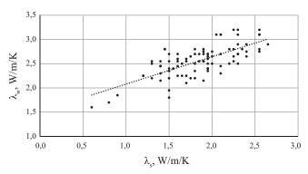
Fig. 2. Collection 1. Linear correlation between the measured values of  $\lambda s$  and  $\lambda w$ . The linear regression equation (line):  $\lambda_w = 1.52 + 0.56 \, \lambda_s \, (R^2 = 0.51, \, N = 90)$ . The standard deviation of individual values of  $\lambda_w$  from the regression line is 0.26 W/m/K. Hereinafter,  $R^2$  is a parameter characterizing the degree of reliability of linear approximation; N is the number of samples
