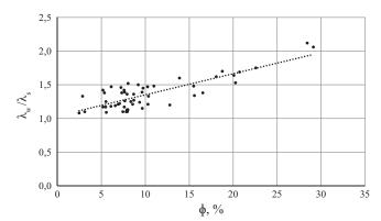
Fig. 3. Collection 1. Linear correlation between the values of the ratio of thermal conductivity of water-saturated and dry samples  $(\lambda_w/\lambda_s)$  and their porosity. The linear regression equation:  $\lambda_w = 1.04 + 0.03 \phi (R^2 = 0.69; N = 54)$
