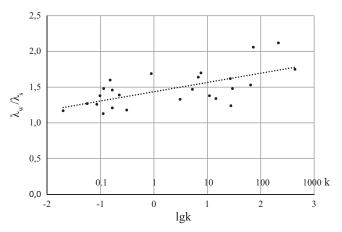
Fig. 4. Collection 1. Linear inverse correlation between the measured values of thermal conductivity of samples  $(\lambda_{u}/\lambda_{v})$ and their permeability (k in mD; lgk). Regression equation:  $\lambda_w/\lambda_s = 1.44 + 0.13 \cdot lgk \ (R^2 = 0.41; N = 25)$
