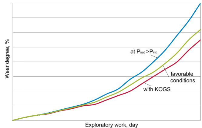
Fig. 6. The dependence of the wear degree on the exploratory work and operating conditions of PCP units
