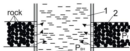
Fig. 1. Gas flow from the oil formation to the well
