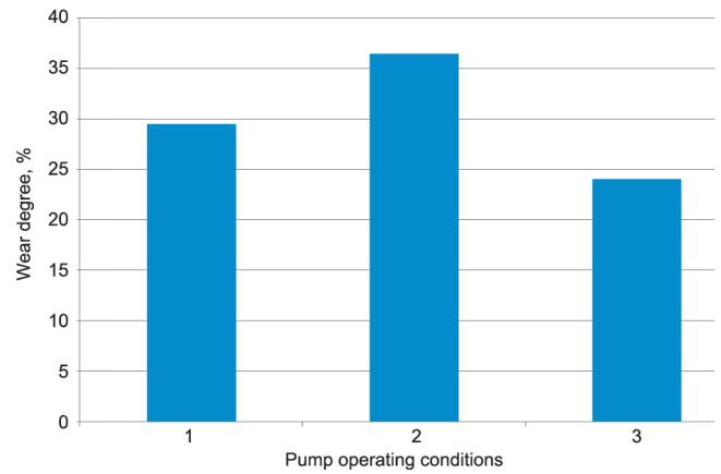
Fig. 5. The wear degree of PCP unit depending on the operating conditions: 1 – favorable, 2 – at  $P_{sat} > P_{in}$ , 3 – with use of KOGS
