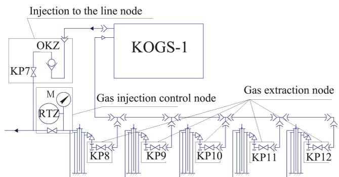
Fig. 4. Layout of a KOGS unit connection in a well cluster: KP7, KP8, KP9, KP10, KP11, KP12 – ball valve, OKZ – check valve, RTZ – pressure sensor, M – pressure gauge
