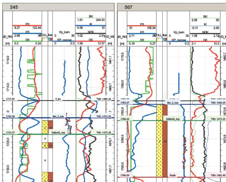
Fig. 6. Well logging board with core sampling intervals in the basal and bar reservoirs
