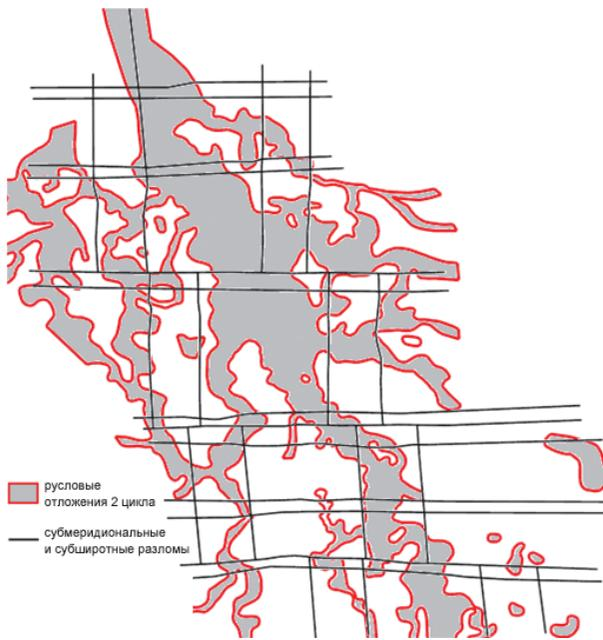
Fig. 10. Distribution map of channel sediments along the area with the imposition of submeridional and sublatitudinal faults
