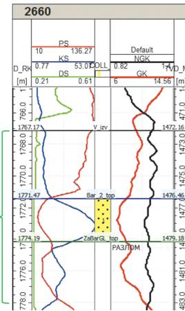
Fig. 5. The fourth type of the section (tidal channel)
