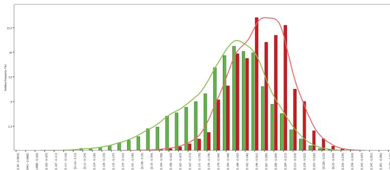
Fig. 8. Comparison of K<sub>p</sub> determined by well logging in basal-bar and channel sediments
