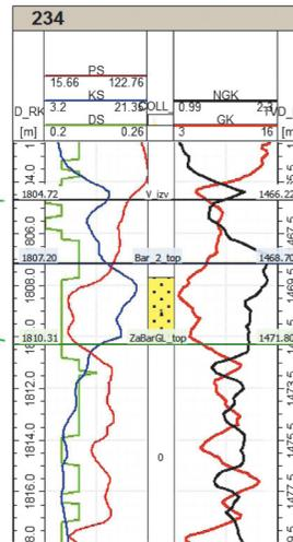
Fig. 3. The second type of the section (channel + basal layer + bar)
