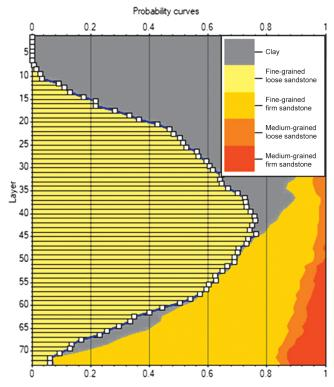
Figure 7. Vertical proportion curve
